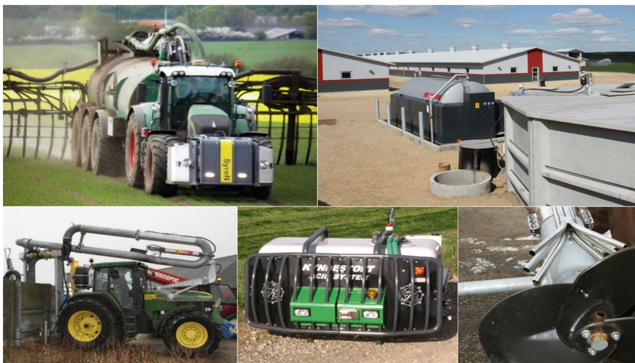
Picture 1: Slurry acidification technologies comprise in-field, in-house, and in-storage technologies.
